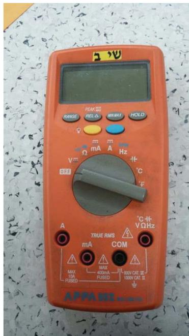
Figure 5. A calibrated APPA 90 Series II Multimeter was used to measure the target object and tarmac temperatures
